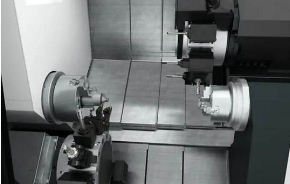
The two spindles and multiple turrets enable efficient 6-sided complete machining of workpieces up to \varnothing 430 \times 700 mm.
