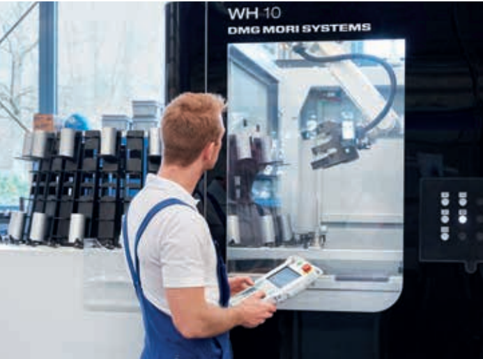
The handling system of the NLX 2500 is designed for workpieces weighing up to 12 kg.
