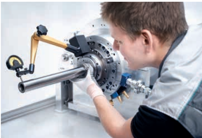
18 hours of geometry checks on the machine and spindles.
