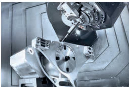
toolcraft manufactures complex precision components like this wheel bearing with highly accurate and productive 5-axis machining.
