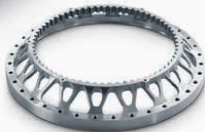
Brake disc housing Turned on a CTX beta 800 Milled on a DMU 80 eVo linear Material: Titanium Duration: 5-axis milling approx. 7 hours
