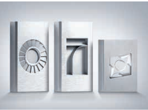
Laser machining of recessed 3D contours in carbide with a picosecond laser.
