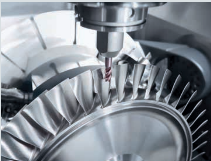
The maximised stability and dynamics of the monoBLOCK® range are ideal for machining blisks.
