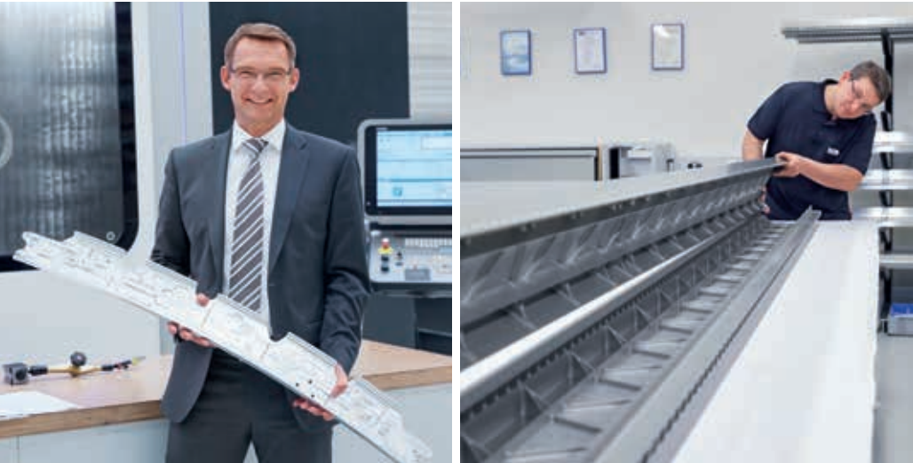
Jens Loll, Managing Director of Loll Feinmechanik, with an aerospace structural component manufactured on a DMF travelling column milling machine from DMG MORI. The dynamics and positioning accuracy of the linear technology help Loll Feinmechanik to machine large workpieces.
