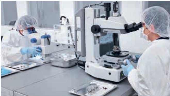
Now at Wernau: MR sensor adjustment to exactly 2 µm by microscope.
