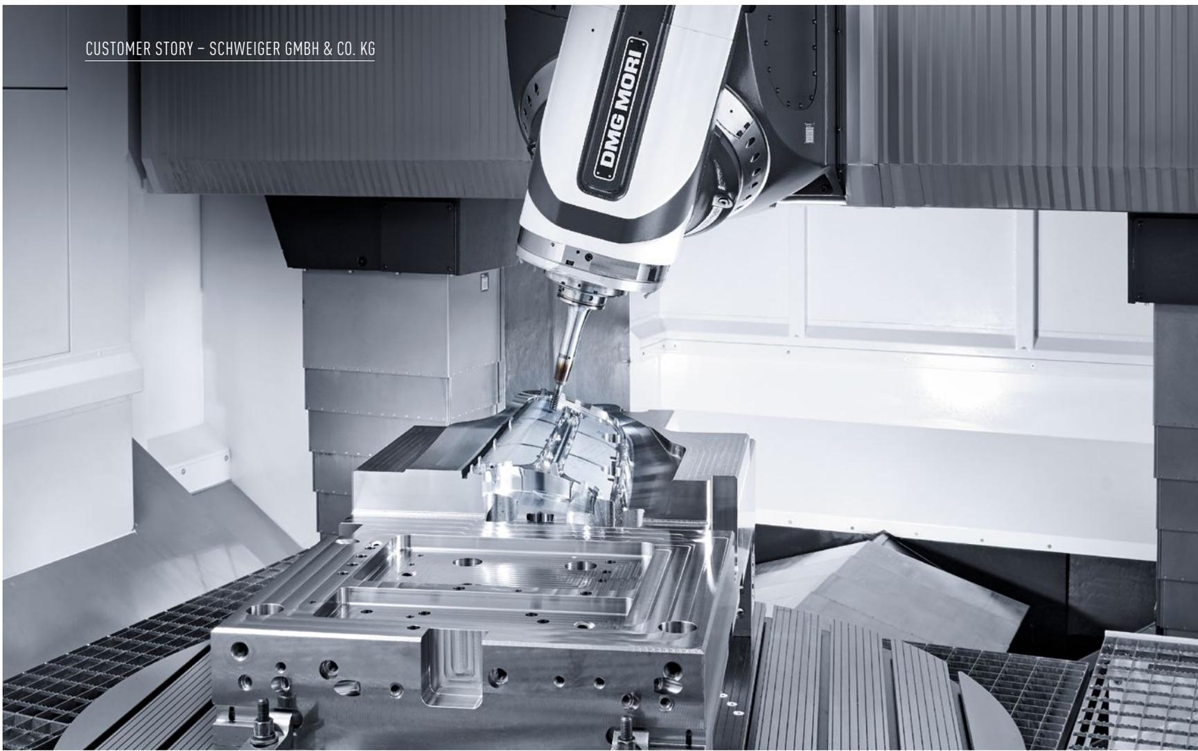
High-precision mold machining on a DMU 210 P.
