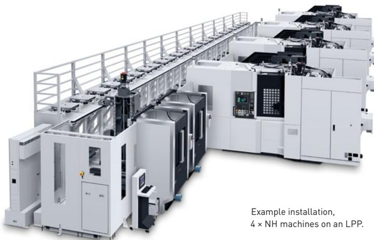
Example installation, 4 x NH machines on an LPP.
