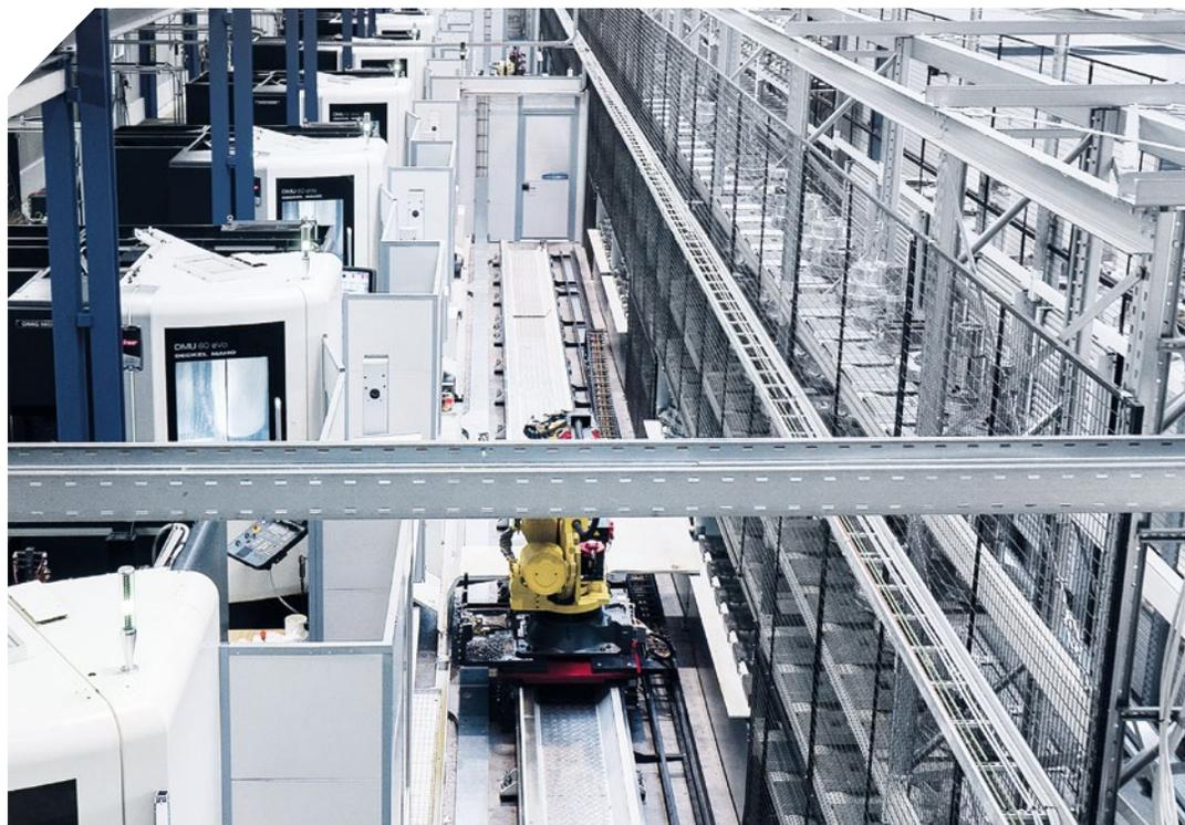
Twelve DMU 60 eVo *linear* machines are linked at PFW via a pallet storage system with 743 locations.
