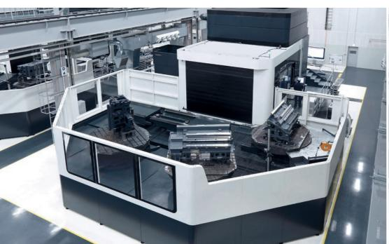
The automated machining of machine beds for the NLX series is carried out on three DMC 340 FD machining centers from sister plant, DECKEL MAHO Pfronten GmbH. Six older gantry machines were replaced with the three mill-turn centers.
