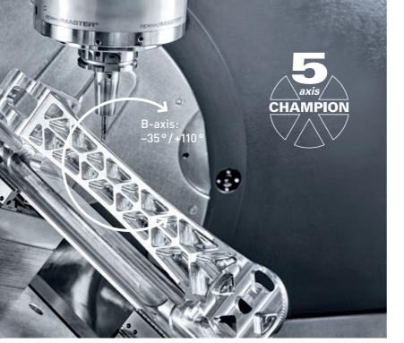
Swivelling rotary table for 5-axis simultaneous machining of workpieces up to 300 kg.
