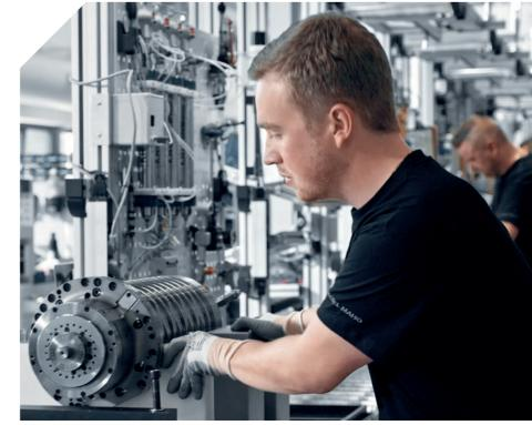
Spindle repair in the DECKEL MAHO
