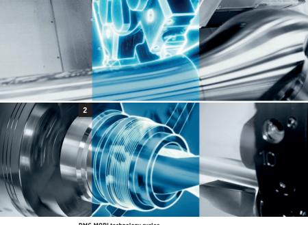
DMG MORI technology cycles 1. Variation of speed: Avoidance of vibration and chatter by modifying the spindle speed 2. Easy Tool Monitoring 2.0: Avoidance of damage following tool breakage or tool overload
