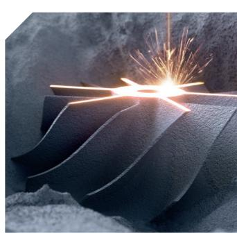
The LASERTEC 30 SLM offers a build volume of 300 × 300 × 300 mm within which any workpiece shapes can be additively manufactured.
