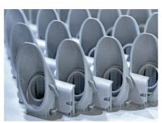
Functional surfaces such as this internal radius are finished accurately in a final machining process.
