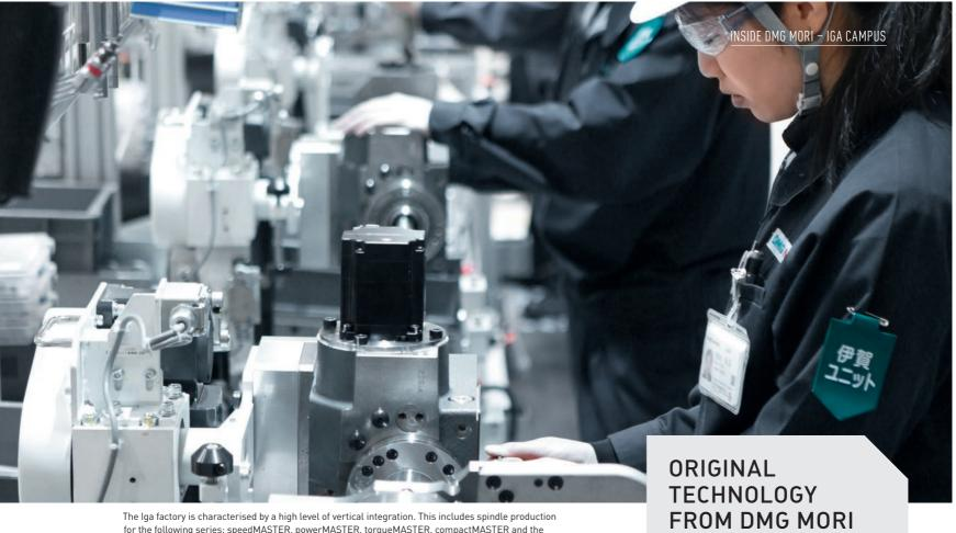
for the following series: speedMASTER, powerMASTER, torqueMASTER, compactMASTER and the turning spindle turnMASTER. Iga produces around 7,000 high-tech spindles a year.
