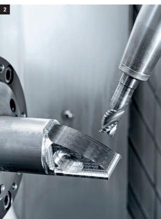
$\textbf{1.-3.} \ \textbf{The stability and cutting performance of DMG MORI machines enable high-precision}$ machining of the complex prosthesis components from aluminium, steel or titanium. 4. Larus Gunnsteinsson, Product Designer
