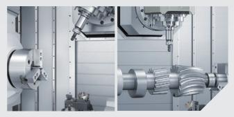
6-sided complete machining of complex workpieces up to ø 670 mm and 1,540 mm in length with the compactMASTER turn & mill spindle and second tool carrier (lower turret) with 80 mm Y-axis.
