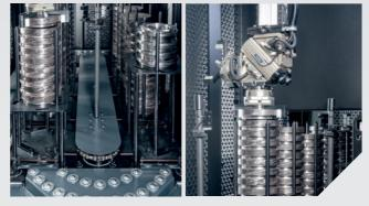
Unmanned production possible due to 10-fold stacking magazine (max.  $10 \times 70$  kg) for workpieces up to  $\emptyset 200 \times 150$  mm and max. 6 kg.
