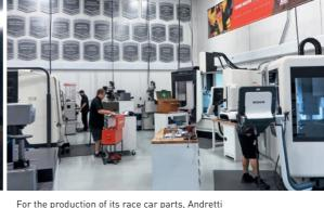
For the production of its race car parts, Andretti Autosport relies on turn-and-mill technology from DMG MORI, namely (from left to right) the NLX 2500 SY | 700, a CMX 1100 V and a DMU 50.
