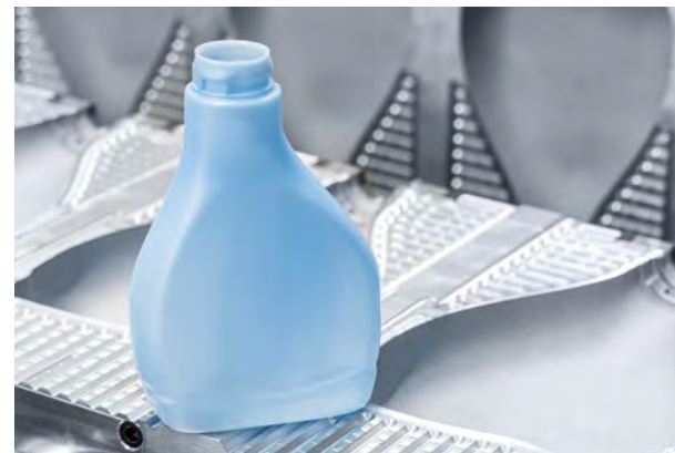
Using a total of 11 DMG MORI machines, Seriomould manufactures high-precision molds for producing plastic bottles, e.g. for food or personal care.
