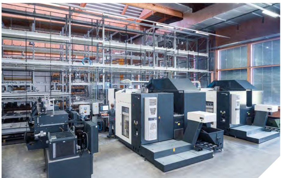
Two DMC 60 H linear machines are connected to the 100-position pallet storage system. Together with the 303-pocket tool magazine, this ensures autonomous production overnight and at weekends.
