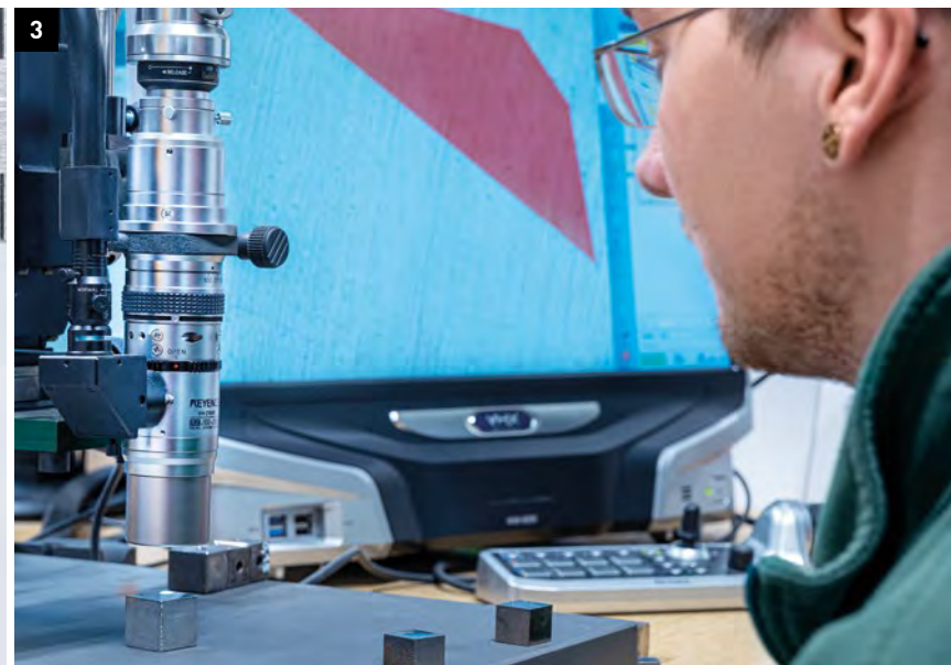
1. The workpieces are programmed externally and transferred to the CELOS APP RDesigner. User-friendly CAM programming from the CAD data is carried out. 2. Even the most filigree geometries can be realized effortlessly in the powder bed process. 3. Modellbau Clauss uses a microscope to check the structural density of the workpieces created in the powder bed.
