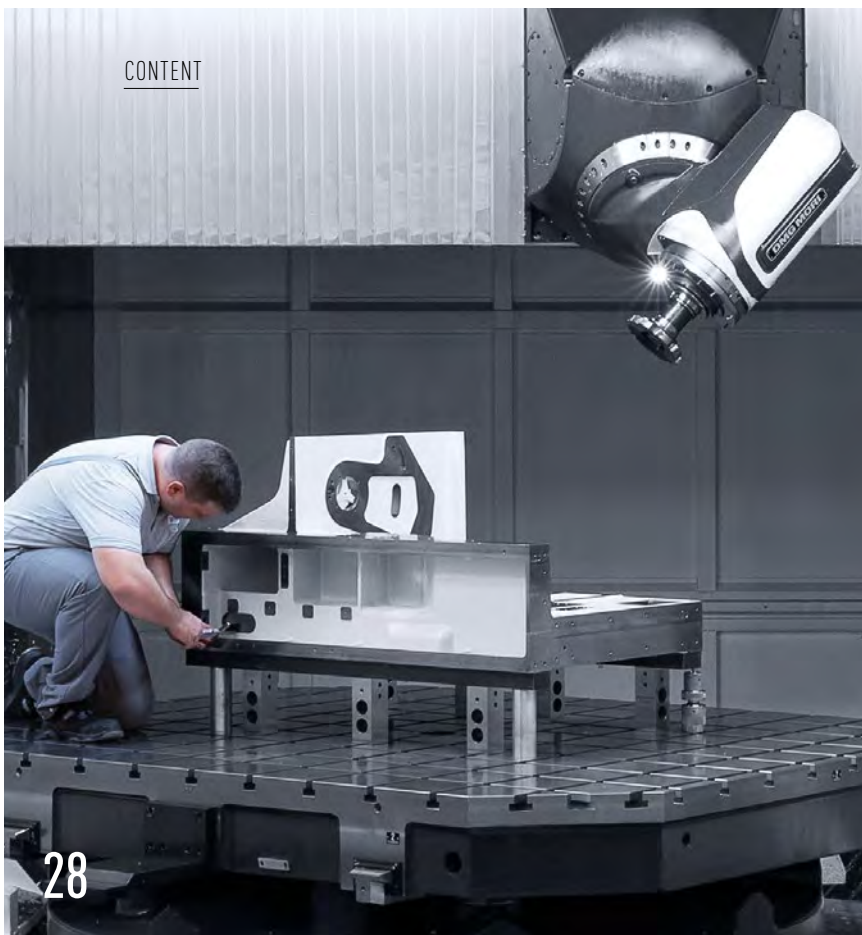
Baltic Metalltechnik: 45 machines from DMG MORI for precision machining down to tens of microns, including a DMC 340 U for large parts up to 3 m.
