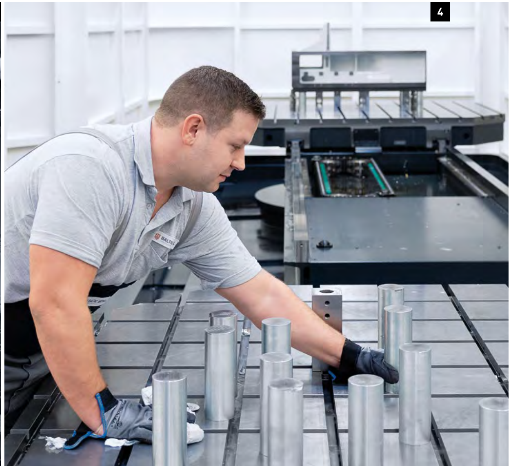
1. Thorsten Deumlich, Head of Large Part Machining at Baltic Metalltechnik GmbH 2./3. Complex, high-precision machine components are produced in 5 axes for the Hauni Group on the DMC 340 U. 4. Operator Marc Hänel sets up workpieces for machining, a process that is simplified using a bespoke table with special slots.
